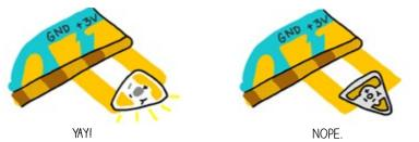
**3. Is there enough overlap between the pads of your LED and the copper tape?** There needs to be plenty of overlap between the metal pad of your LED and the copper tape for there to be a strong electrical connection. If the overlapping area is too small, then power can not flow to the LED.
