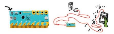
**2. Is the PWR light red instead of green?** That typically means we have a short circuit connecting +3V and GND directly to each other, draining power from the Chibi Chip! If you're powering the Chibi Chip from a computer, an error message may also pop up on your screen about too much power or current being drawn.
