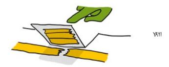
14. Is the switch sometimes working and sometimes not when pressed? That means the switch connection is unreliable. Check that the copper tape is smooth and clean on both halves of the switch. Then, try ways to increase the pressure between the pieces of copper tape in your switch.
