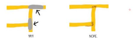
**12. Do you have a moving hinge in your circuit?** Make sure to reinforce it with a conductive fabric patch. Tears are especially common at places where the copper tape gets folded repeatedly. Copper tape will crack when folded too many times.
