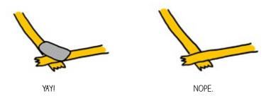
Make reliable turns with a single piece of copper tape and save on conductive fabric patches using this origami trick:
