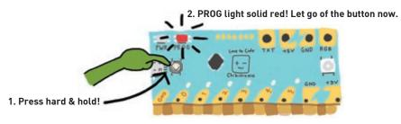
**7.** Is the Chibi Chip hearing the audio code? During upload, the red PROG light on the Chibi Chip should blink to show that it hears the code. If the PROG light stays solid red, even though the sound should be playing, it means the audio is not making it to your Chibi Chip. If this is the case, try turning up the volume on your device and check that sounds are playing (**Step 3**).
