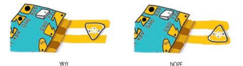
**2. Are any LEDs causing a short circuit?** Make sure that the shiny metal pads of your LEDs are touching only one strip of copper tape. If one pad of an LED is touching two different copper wires, then there is a short circuit and your light will not turn on. In the example below on the right, the wide (+) side is accidentally touching both GND and +3V, causing a short circuit!
