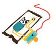
Here's what the finished pocket character switch looks like. When we put the cat in the pocket, it will close the circuit, turning the switch on. Make sure to push the cat all the way into the pocket for a secure connection.
