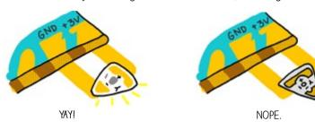
**3.** Is there enough overlap between the pads of your LED and the copper tape? There needs to be plenty of overlap between the metal pad of your LED and the copper tape for there to be a strong electrical connection. If the overlapping area is too small, then power can not flow to the LED.
