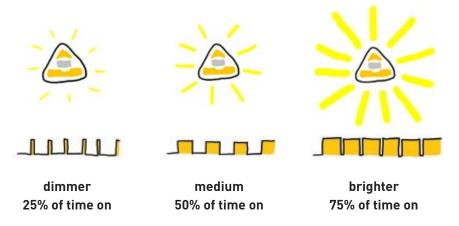
There's a trick you can try to see the blinking for yourself. First, program a LED to fade and then wave it very quickly in front of your eyes. Instead of seeing a continuous streak of light, you will see a "dotted line" of light. This is the light turning on and off very rapidly! Next, fix the light to on, by programming it using on() and try waving it around again. This time, you'll see a continuous, solid streak!
