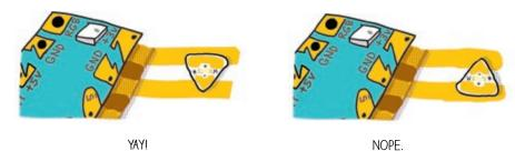
2. Are any LEDs causing a short circuit? Make sure that the shiny metal pads of your LEDs are touching only one strip of copper tape. If one pad of an LED is touching two different copper wires, then there is a short circuit and your light will not turn on. In the example below on the right, the wide (+) side is accidentally touching both GND and +3V, causing a short circuit!
