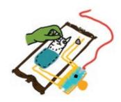
We can turn off the switch by pulling the cat out of the pocket, or by flipping the cat around so that the copper tape doesn't touch the circuit.
