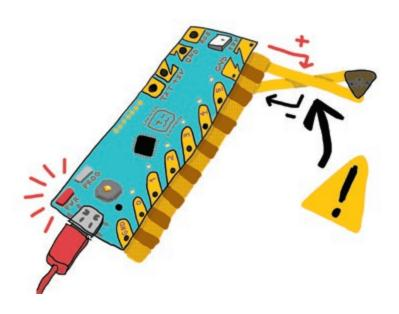
If this happens to a Chibi Chip, the Chip will shine a red warning light until the short circuit is disconnected.
