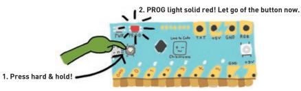
7. Is the Chibi Chip hearing the audio code? During upload, the red PROG light on the Chibi Chip should blink to show that it hears the code. If the PROG light stays solid red, even though the sound should be playing, it means the audio is not making it to your Chibi Chip. If this is the case, try turning up the volume on your device and check that sounds are playing [Step 3].
