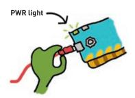
**1. Is the PWR light off?** If so, it means the Chibi Chip is off because it isn't getting enough power! Try plugging the Chibi Chip into a power supply that you've recently used to charge a phone, like a USB wall plug or computer's USB port. Phones take a lot of power to charge, so if the USB port can charge a phone, it can power a Chibi Chip!
