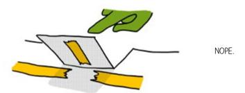
Make the copper tape patch large and the circuit gap small. This makes it easier for your switch to close the circuit. This is especially important for more advanced switches, such as the wind sensing switch (page 3-28), where the switch isn't actually pressed by hand.
