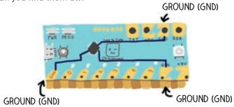
Even though they look like three separate pins, they are actually connected together by copper traces inside the Chibi Chip. This means that they are all at the same voltage (0 volts) so connecting to one ground pin is the same as connecting to another ground pin.
