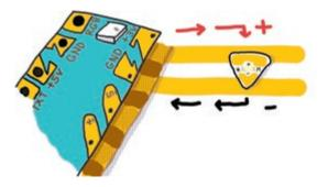
Clipping on the Chibi Chip makes a complete circuit! This means that everything got connected in an unbroken loop that allows power to flow, turning on the LED light.
