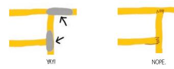
**12. Do you have a moving hinge in your circuit?** Make sure to reinforce it with a conductive fabric patch. Tears are especially common at places where the copper tape gets folded repeatedly. Copper tape will crack when folded too many times.
