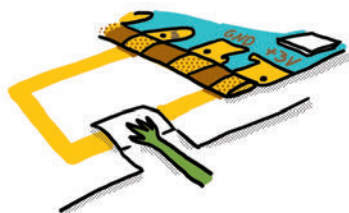
pin 5 connected to +3V pressed
